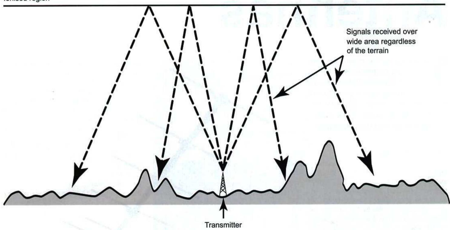
Near-vertical incidence skywave gives propagation for a radius of 100 miles or more by reflecting signals more or less straight down from the ionosphere (as opposed to the small angles of reflection used for DX working).
