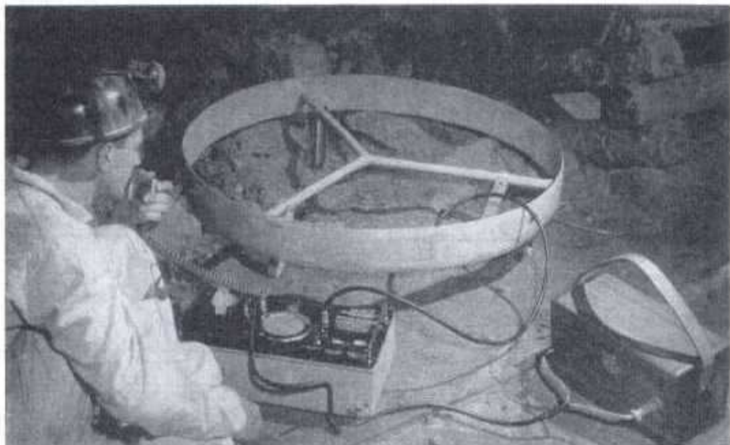
Fig. 3. The base station and its wagon-wheel antenna c. 1960
