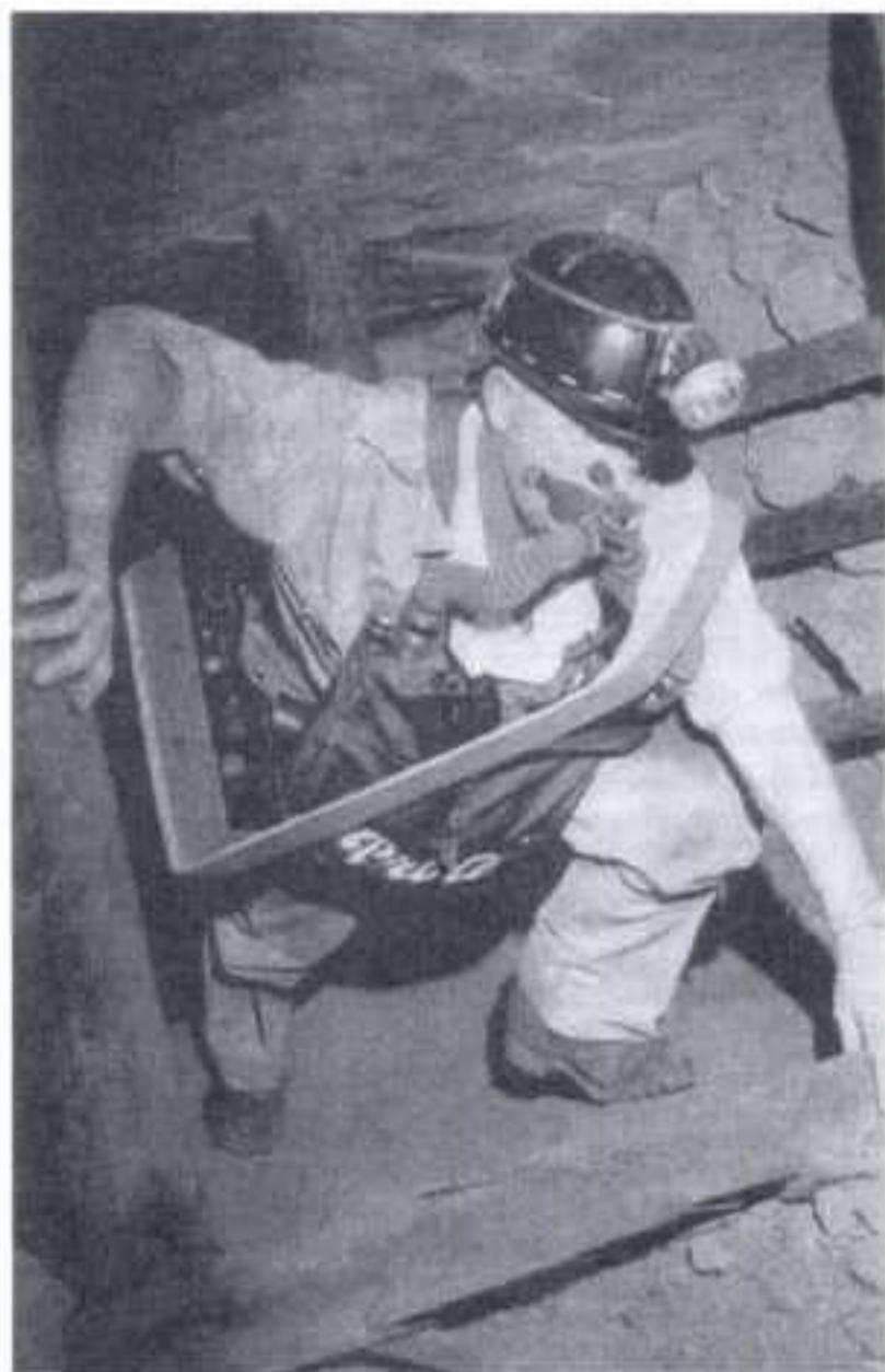
Fig. 4. The portable equipment used by a rescue brigadesman wearing breathing apparatus, mouth-piece and nose clip
