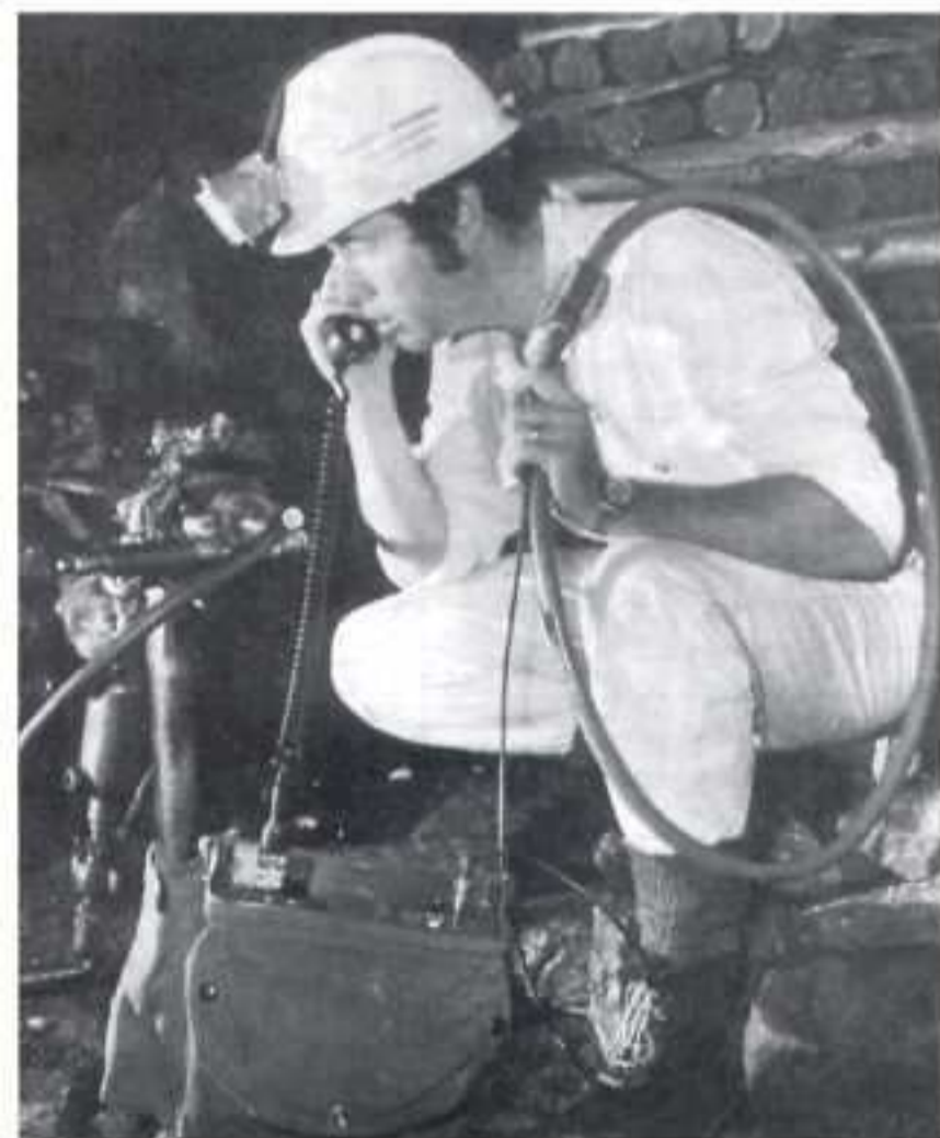
Fig. 6. The 335kHz solid-state 10W SSB transceiver and elliptical loop antenna c.1972
