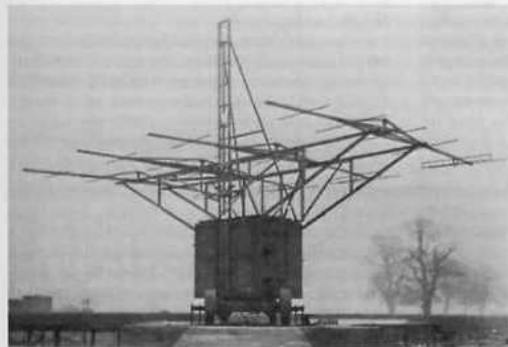
GLII fitted with an array of four Yagi antennas
