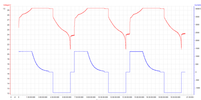
Figure 5: Test Charge - Discharge Cycle
